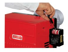
Head setting is easy and aided by a graduated scale, a test point allows reading the air pressure in the combustion head.
